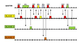
Fig. 2: Bluetooth working Procedure
