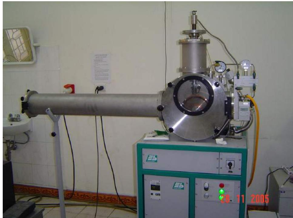
**Fig.3. Vacuum arc melting machine**
